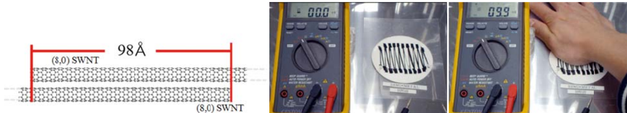
Fig. 1: (a) The laterally-contacted SWNTs. (b) Demonstration of an SWNT thermoelectric device. [7]
